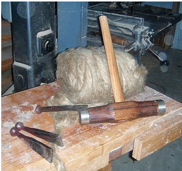
All the tools you need to caulk the deck seams. This is a caulking mallet, caulking irons and a bundle of oakum. You would roll this into thinner strips first.
