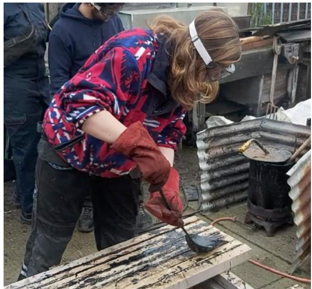
A boatbuilding student practices her skills on a pretend piece of deck. Here you can see how the tar is poured over the seams between the deck planks.
